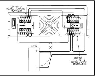
Figure 4-14. Series Connections with Remote Sensing
